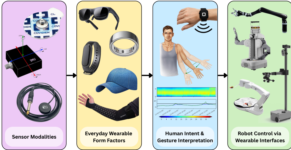
Figure 1: An overview of the pipeline to use sensors as robot control interfaces: Diverse sensing modalities such as EMGs, IMUs, and contact microphones are embedded into everyday wearable form factors such as glasses, rings, wristbands, hats and sleeves. They capture user motion and physiological cues that are then processed to infer human intent and gestures, enabling robots to execute tasks through wearable control interfaces.
